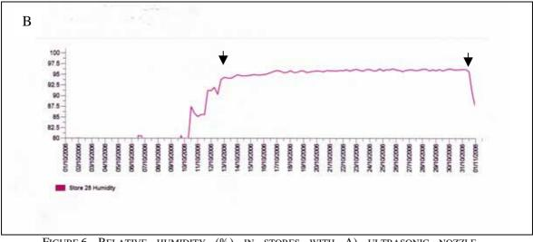
Figure 6 Relative humidity (%) in stores with A) ultrasonic nozzle humidifier; and B) Munters HM2 4000 evaporative humidifier.
