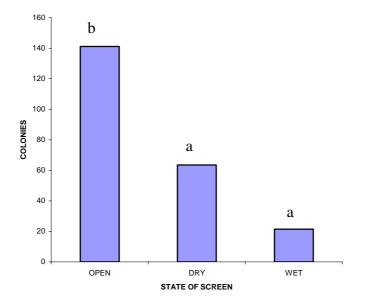
FIGURE 3 THE NUMBER OF COLONY FORMING UNITS RECOVERED ON PETRI DISHES POSITIONED BEHIND THE HUMIDIFIER UNIT WITH HUMIDIFIER SCREEN REMOVED (OPEN); SCREEN INSTALLED DRY; AND SCREEN INSTALLED WET (I.E. NORMAL OPERATION). LSD<sub>(P=0.05)</sub> = 49 (14 df). Different letters above the columns indicate a significant difference at P<0.05.
