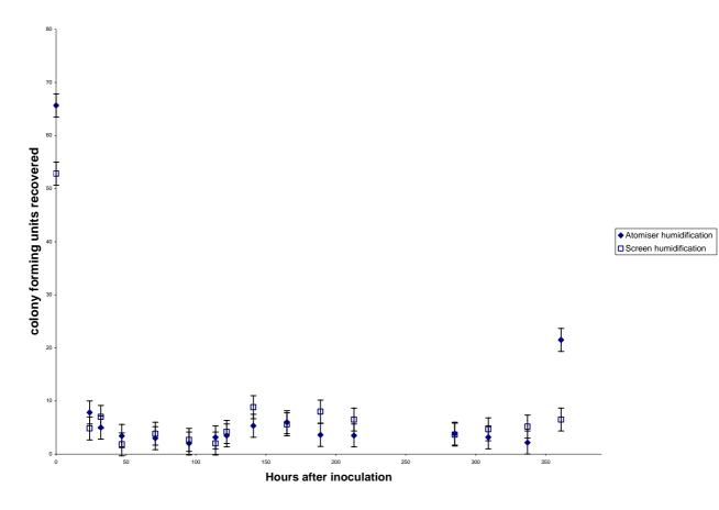
FIGURE 7 NUMBER OF FUNGAL COLONY FORMING UNITS RECOVERED OVER A 15 DAY PERIOD FROM TWO EXPERIMENTAL STORES (ONE, WITH ATOMISER HUMIDIFICATION; THE OTHER WITH SCREEN HUMIDIFICATION).
