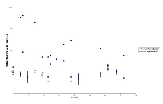
FIGURE 8 NUMBER OF BACTERIAL COLONY FORMING UNITS RECOVERED OVER A 15 DAY PERIOD FROM TWO EXPERIMENTAL STORES (ONE WITH ATOMISER HUMIDIFICATION; THE OTHER WITH SCREEN HUMIDIFICATION).
