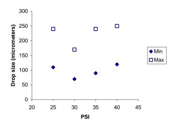
Figure 1 The relationship between the size of water droplet produced by airbrush and air pressure.
